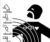
ELECTRIC AND MAGNETIC FIELDS - May be dangerous. Electric current following through any conductor causes localized Electric and Magnetic Fields (EMF). Welding/cutting current creates EMF fields around cables and power sources.
