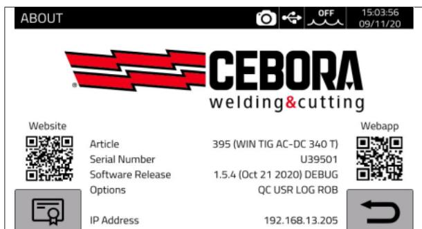
During start-up, for 5 seconds the display presents all the information regarding the machine, the serial number, the software version, when the software was updated, the options installed and the IP address. The display then presents the main screen (factory setting).
