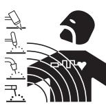
· Electric current flowing through any conductor causes localized Electric and Magnetic Fields (EMF). Welding/cutting current creates EMF fields around cables and power sources.
