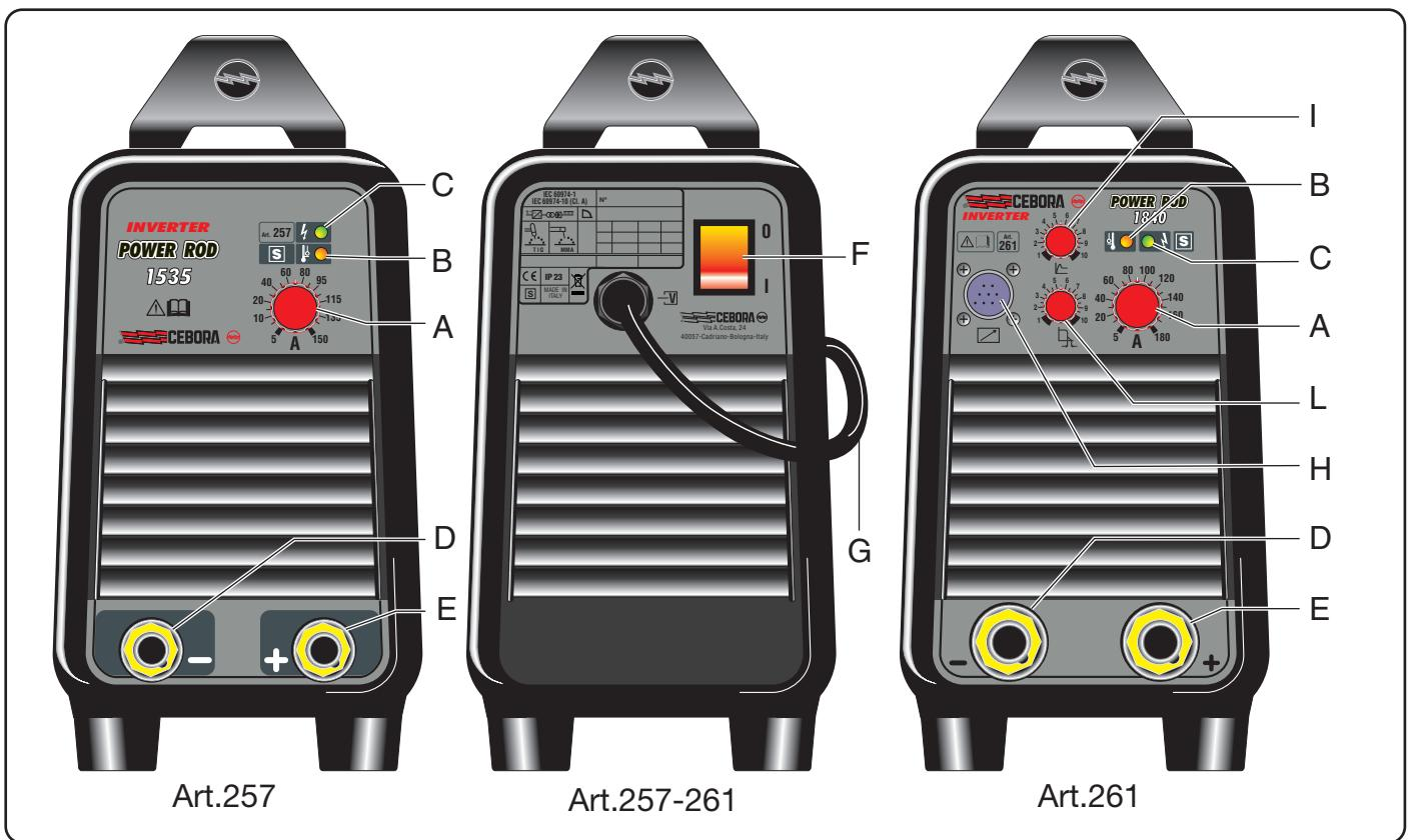
I) Adjusts an overcurrent that may be inserted to aid in striking the arc. This function is active in both MMA and TIG modes (Art. 261).
