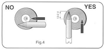
CAUTION. HOT FLYING METAL PARTICLES can injure personnel, start fires, and damage equipment: TUNGSTEN CONTAMINATION can lower weld quality.
