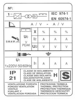
IEC 974.I. The welder is manufactured according to this EN 60947.1 international standard.
