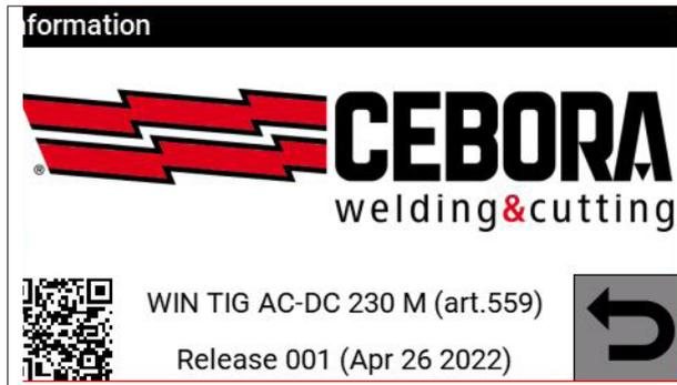
During start-up, for a few seconds the display presents all the information regarding the machine item number, the serial number, the software version, and when the software was updated.
