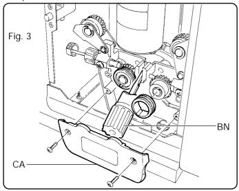
Open the door **BJ**, remove the cover **CA**, release the wire press rollers using the pressure setting knob **BN**, replace the rollers and remount the cover **CA**.
