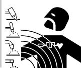
ELECTRIC AND MAGNETIC FIELDS - May be dangerous. Electric current following through any conductor causes localized Electric and Magnetic Fields (EMF). Welding/cutting current creates EMF fields around cables and power sources.
