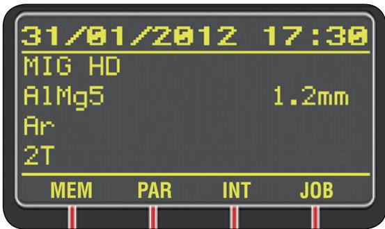
The program parameters are changeable using the normal editing process, **T7 (PAR)**.
