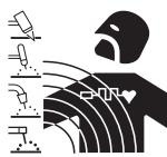
· Electric current flowing through any conductor causes localized Electric and Magnetic Fields (EMF). Welding/cutting current creates EMF fields around cables and power sources.
