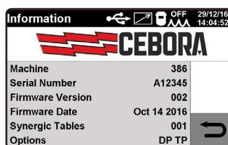
When the machine is switched on, for a few moments the display shows: the article number of the machine, the serial number, the Firmware version, the date of the Firmware development and the release number of the synergic curves table and the power supply options.
