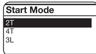
Mode **3L** Specially well suited to weld aluminium.
