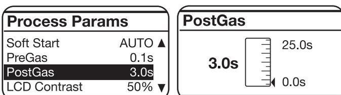
The adjustment can vary from 0 to 25 seconds.
