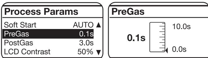
The adjustment can vary from 0 to 10 seconds.
