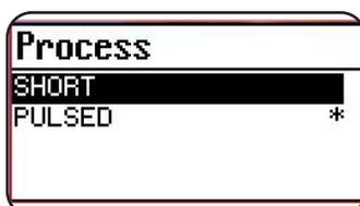
Use knob **B** to choose or confirm a welding mode by selecting and pressing **Short** or **Pulsed** for at least 2 seconds.
