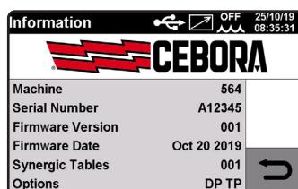
The display shows: Machine item number, serial number, firmware version, firmware development date and release number of the synergic curve table and the installed options.
