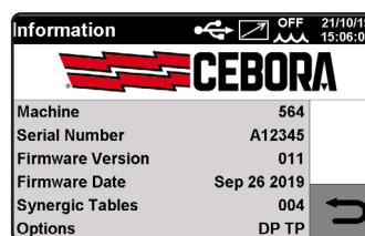
When the machine is switched on, for a few moments the display shows: the machine item number, the serial number, the firmware version, the firmware development date and the release number of the synergic curve table and power source options. This information is also given in menu **(i)**.
