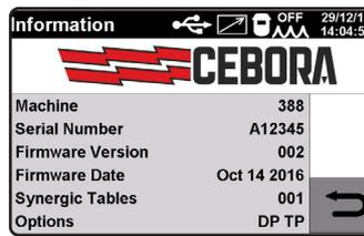
When the machine is switched on, for a few moments the display shows: the article number of the machine, the serial number, the Firmware version, the date of the Firmware development and the release number of the synergic curves table and the power supply options. This information is also given in menu **1**.
