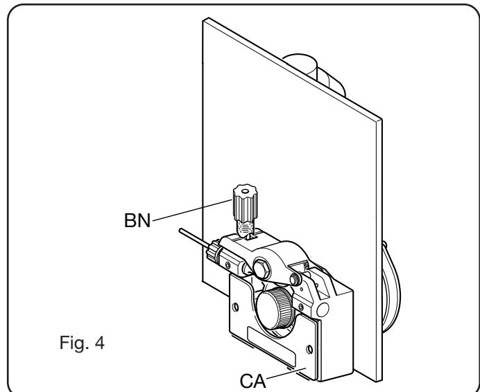
Mount the wire coil and slip the wire into the feeder and welding torch sheath.
