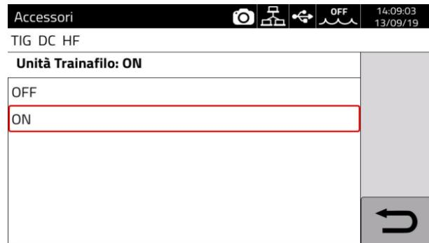
The cold wire feeder is now activated and the operating mode can be selected:
