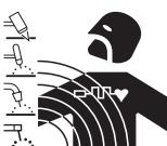
· Electric current flowing through any conductor causes localized Electric and Magnetic Fields (EMF). Welding/cutting current creates EMF fields around cables and power sources.
