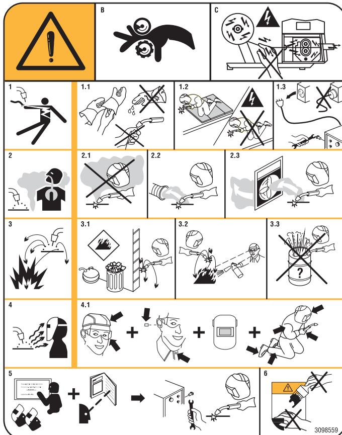
1. Electric shocks caused by the welding electrode or cable can be fatal. Protect yourself properly against the danger of electric shocks.
