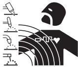
The magnetic fields created by high currents may affect the operation of pacemakers. Wearers of vital electronic equipment (pacemakers) shall consult their physician before beginning any arc welding, cutting, gouging or spot welding operations.
