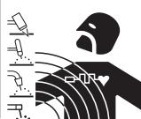
ELECTRIC AND MAGNETIC FIELDS - May be dangerous. Electric current flowing through any conductor causes localized Electric and Magnetic Fields (EMF). Welding/cutting current creates EMF fields around cables and power sources.
