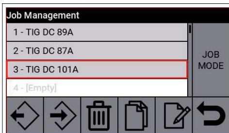
Select the memory position of the JOB to be used, turning encoder **B**.
