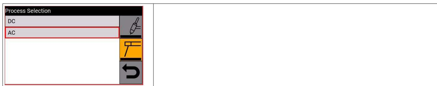
In the MMA AC this process, the output current frequency is 50 Hz and the output waveform is square. Frequency and waveform are fixed and unmodifiable, unlike the TIG AC process.
