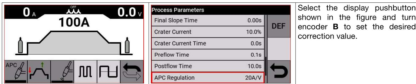
The correction value can be set from the main screen or in the **Process parameter** menu: **Z key -> APC Regulation**
