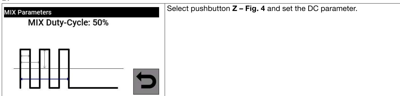
Set the Duty-Cycle Mix parameter to define the direct current penetration percentage within the **AC welding period**. The alternating component parameters are defined in section **V of the display**.
