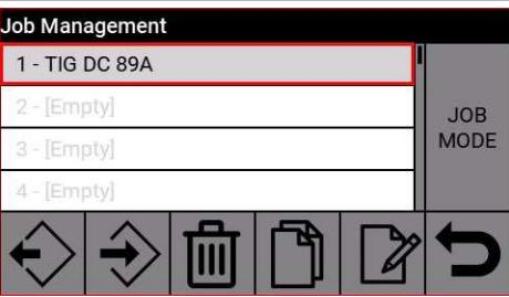
Choose the memory position where the job is to be saved and confirm by pressing encoder B. A description of the saved process will now appear.
