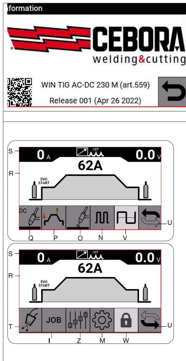
During start-up, for a few seconds the display presents all the information regarding the machine item number, the serial number, the software version, and when the software was updated.
