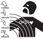
· Electric current following through any conductor causes localized Electric and Magnetic Fields (EMF). Welding/cutting current creates EMF fields around cables and power sources.
