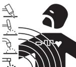
· Electric current following through any conductor causes localized Electric and Magnetic Fields (EMF). Welding/cutting current creates EMF fields around cables and power sources.
