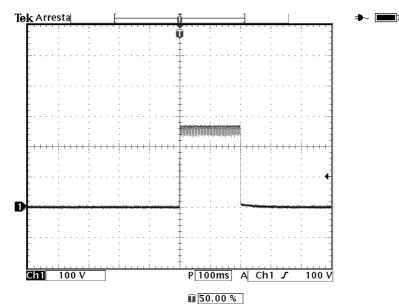
5.2.1 - Power source output voltage, interrupted for missing pilot arc light on (par. 3.3.4).
