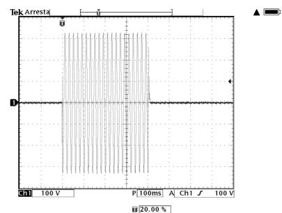
5.2.2 - Solenoid valve ELT (6) voltage supply, interrupted after 400 msec. approximately for missing pilot arc light on (par. 3.3.4).
