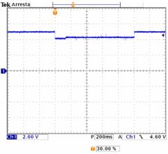
5.2.1 - Reference signal for pilot arc current (par. 3.3.8).
