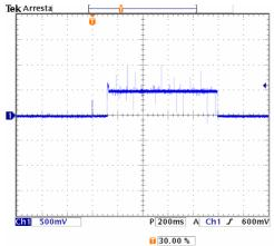
5.2.2 - Feedback signal of the Power Source output current (par. 3.3.8).
