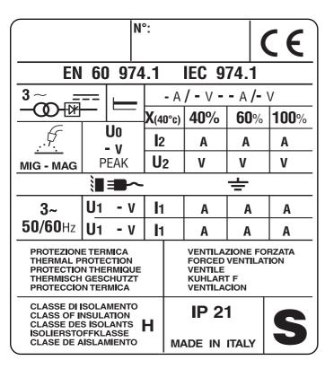
MIG/MAG. Continuous wire welding Uo...... Secondary no-load voltage
