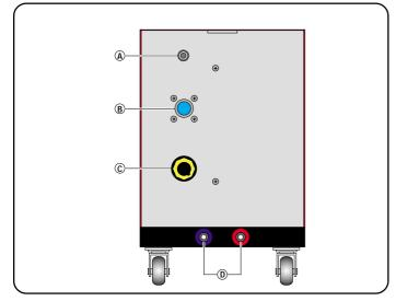
A - Gas hose fitting for extension gas hoses.
