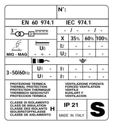
MIG/MAG. Continuous wire welding Uo...... Secondary no-load voltage
