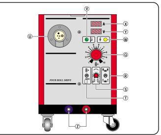
This knob adjusts the wire feed speed. **R- Weld function selection switch** This switch selects among the following functions:
