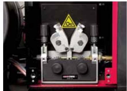
**SOUND MIG 5040/T STAR PULSE** (art. 389) è un **inverter three-phase power source with pulsed** synergic operation, intended for professional use, wherever top-quality welding is required along with high productivity. It is also a multi-process power source, able to weld in MIG-MAG, TIG (contact ignition with "LIFT" system by Cebora) and MMA mode. It is supplied with **integrated torch cooling unit and 4 roller (ø 40 mm) wire feed unit**.
