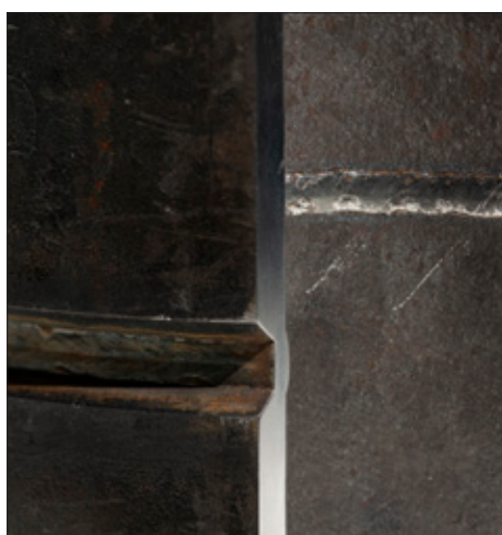
MIG SRS - First pass on tube with bevelling
