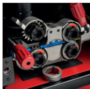
Compact 4-roller quick-release wire feed unit with insertion rollers (ø 37 mm), easily identifiable thanks to color-coding system through diameters
