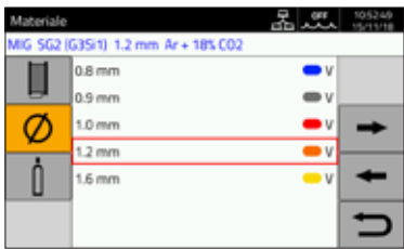
Set-up of the filler wire with indication of the roller type
